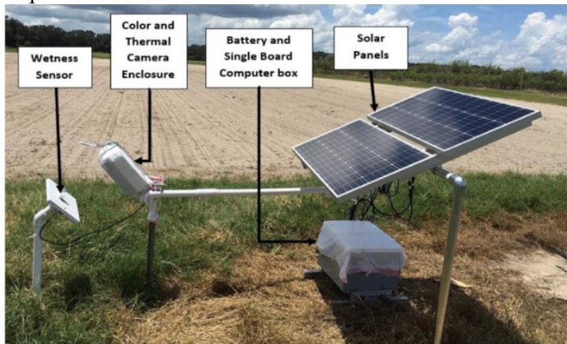
Fig 6 System to monitor wetness sensor using an RGB and infrared camera at UF PSREU, Citra.
